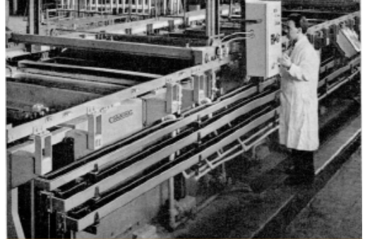
Busbars fitted alongside a Glydo rack plating installation.
