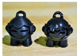
Fig 4: As manufactured and after polishing
