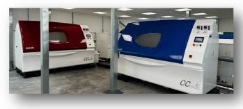
The Oaktree facility houses a number of Ascott Analytical cyclic corrosion chambers. Ranging from the CC450ip, a 450 litre chamber for smaller component parts & small test panel batches to the CC2600ip, a 2600 litre
