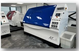
These tests are cyclic in nature and comprise of exposure under controlled and varying conditions of temperature and humidity, with intermittent spraying of a salt solution directly on to the samples under test, from a high level swaying spray bar. The Atmosfär chambers offer additional features compared to the CCip series chambers including:
