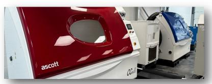
certain metallic, organic, anodic oxide and conversion coatings. Giving an indication to a coating or finish's ability to resist corrosion during its life in service.
