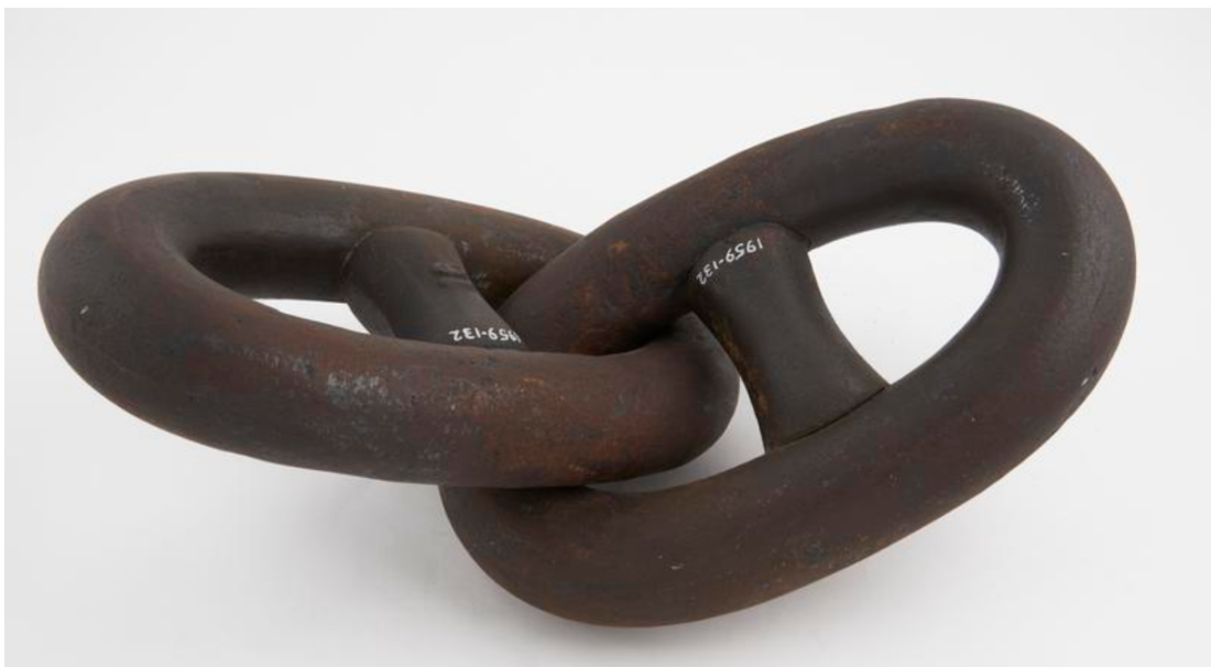
Chain cable made from puddled iron
